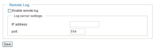
You can configure the Network Camera to send the system log file to a remote server as a log backup. Before utilizing this feature, it is suggested to install a log-recording tool to receive system log messages from the Network Camera. For example, a tool -- Kiwi Syslog Daemon. Visit http://www.kiwisyslog.com/kiwi-syslog-daemon-overview/.
